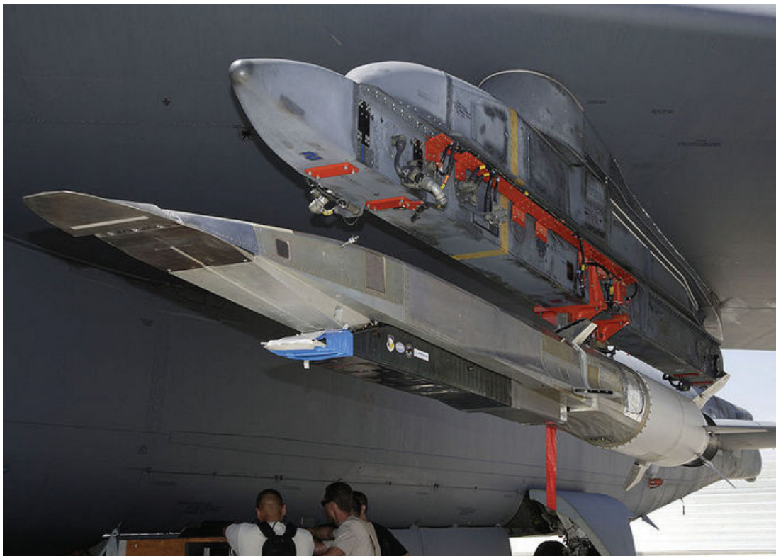
Figure 2 Wave rider type missile configuration: The X-51 Waverider, attached to the underbelly of a B-52 long-range bomber ( Wright-Patterson AFB photo gallery / Chad Bellay / United States Air Force )
